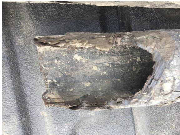
Photo 87 - No-Corrode Sewer Pipe Used for Electrical Cables from Church
